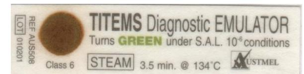
This is a **FAIL**. Emulator will "burn" due to lack of moisture in the steam during sterilization.
