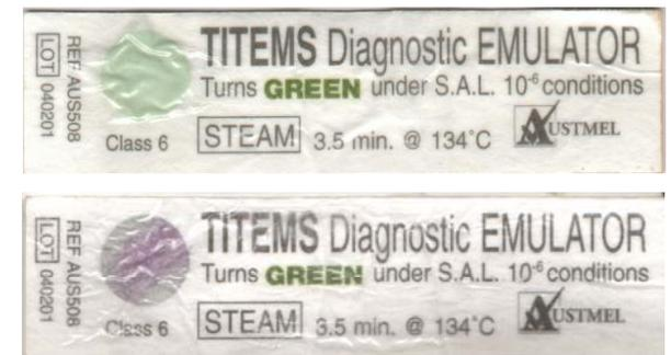
**WET:** Emulator laminate will "bubble" when excessive moisture has been present in the sterilizing process.
